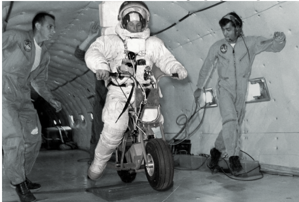
Figure 1. Apollo “Lunar Motorbike”: Testing under simulated lunar gravity (NASA).
